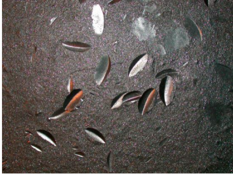
Figure 1.3. Picture of MAX phase Ti_2AlC after hit with a steel hammer; picture's width is about 20cm. Picture courtesy of 3-ONE-2.
